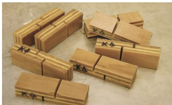
PureBond plywood after ANSI HP-1-2004 cyclic boil test. PureBond's superior moisture resistance approaches Type 1 for waterproof performance.
