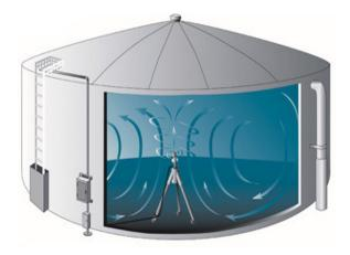
The PAX Water Mixer's Lily Impeller is designed using computational fluid dynamics to reverse engineer the creation of whirlpool flows found in nature. The diagram illustrates the movement the impeller creates.
