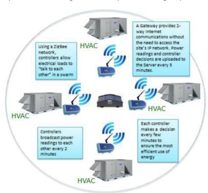
EnviroGrid Controllers record the energy usage of each HVAC system every two minutes and broadcast their readings via a ZigBee network. In this way, the devices act like a swarm of bees.
